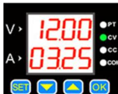
Press "OK" to turn on and off the output. If the load current is below the set current, the output is a constant voltage. The CV light comes on.
