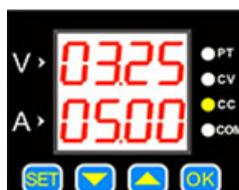
If the load current reaches the set current, the output is at the same level as the set current and constant current. Then the CC light comes on.
