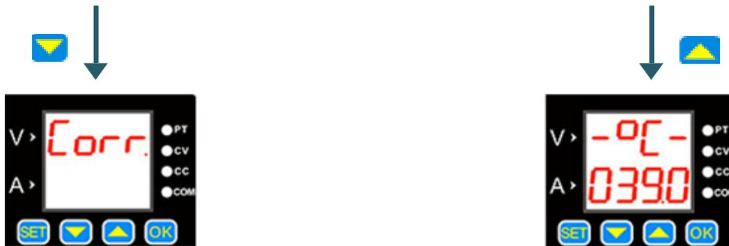
Press **▼** to return to the menu. To calibrate the device press **OK**. In the following is the function of the calibration explained.
