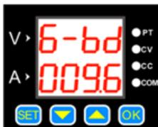
In this menu point you can enter the baud rates. There are 7 different rates in Kbps.
