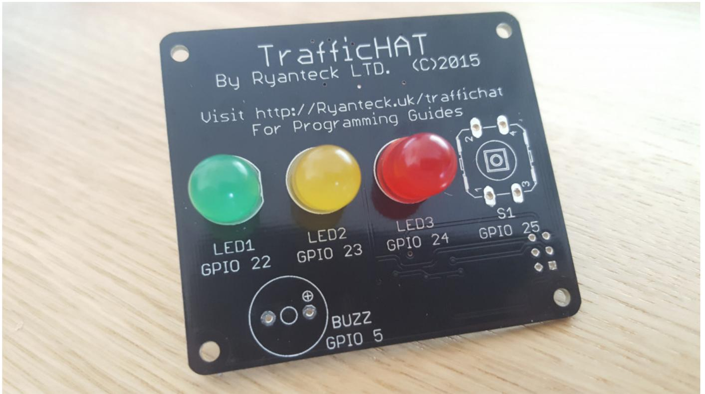
**Note:** You can affix the components in place using some blu tack or by bending the legs of the LEDs before soldering as per the below image
