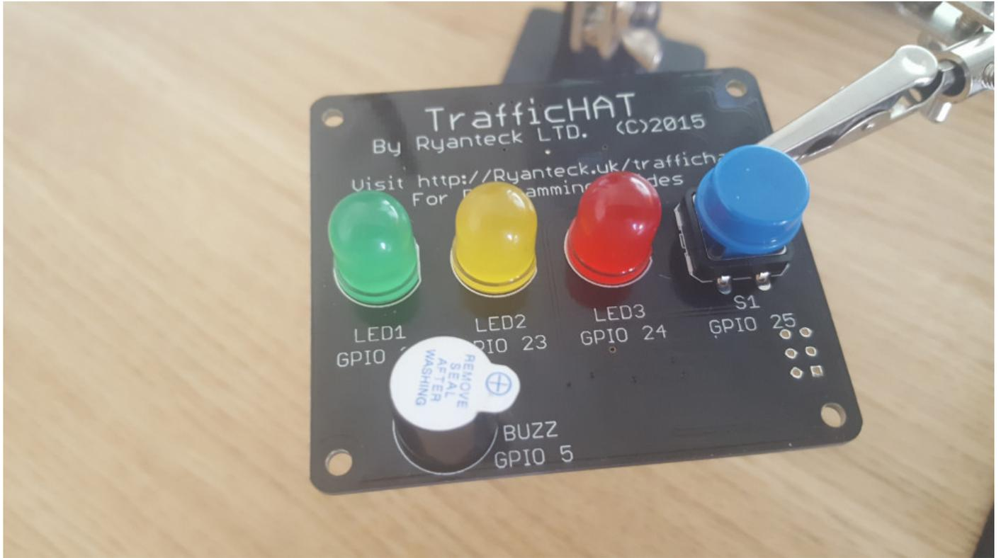
**Step 4** - Now solder all the legs on the underside of the PCB board, making sure you apply enough solder to make good contact between components.
