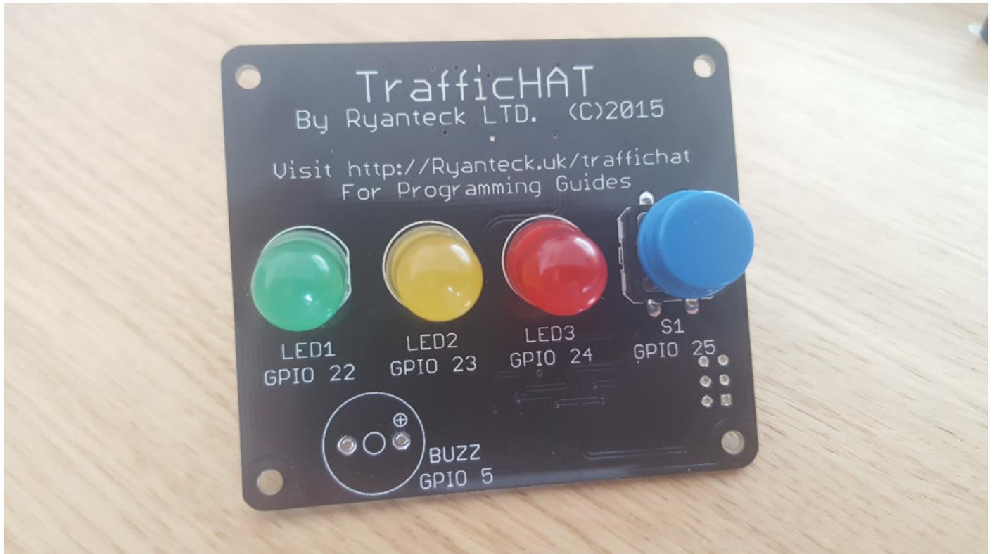
**Step 3** - Lastly, insert the piezo buzzer into the BUZZ through hole solder pads on the Traffic HAT PCB. You can see there is a + symbol to indicate where the positive leg of the buzzer goes through. The positive leg on the buzzer is the longest leg, also indicated by the sticker on the top of the buzzer.
