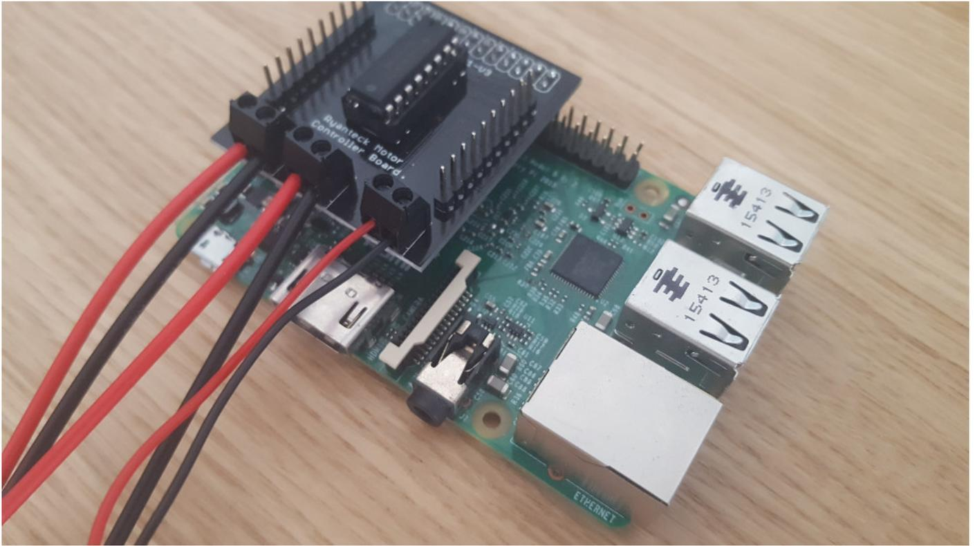
**Step 5** - Boot up your Raspberry Pi by connecting the power supply and also insert the batteries to the motor controller board if you haven't done so already.
