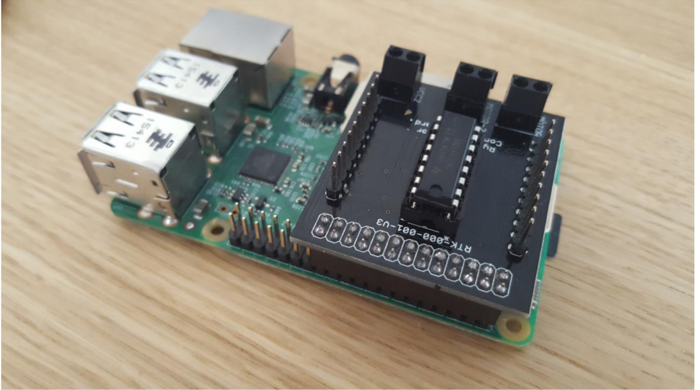
**Step 3** - Insert the wires from the motors into the screw terminals on the motor controller board labelled Motor-1 and Motor-2.
