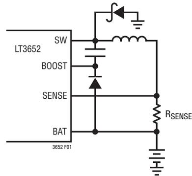
Figure 1. Programming Maximum Charge Current Using  $R_{SENSE}$
