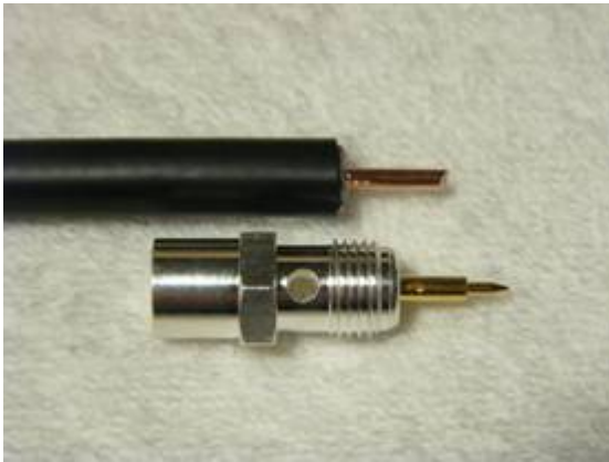
1.Strip center conductor 13mm
