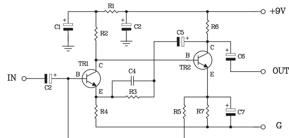
Figure 2. The dynamic microphone preamplifier circuit
