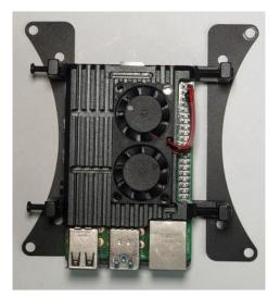
Now you can mount your housing as shown in the picture. The mounting of the case can vary from case to case.
