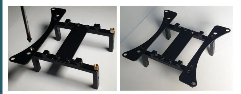
Attach the VESA adapter to the previously screwed-in standoffs using 4 M3 x 5 mm countersunk screws. Make sure that the side of the VESA adapters with the countersink is facing upwards.
