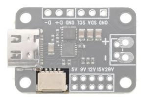
To configure the PD controller and change the output voltage and current limit from a microcontroller, I2C pins are broken out both as individual pins and as a JST-SH 1.0mm QWIIC connector. The PD controller works as an I2C slave on address 0x08. I2C takes priority over the manual voltage setting. External pullup resistors for SCL/SDA must be used.
