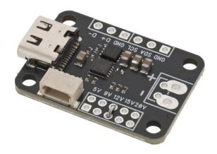
Before use, the module must be configured to request the desired voltage from a connected USB power supply. A 2x5-pin header is included in the package and can be soldered to the board for a quick and easy way to change the voltage using the included jumper. For a more permanent and low-profile application, a simple wire or component lead can be used instead of the entire pin header.
