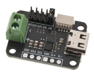
This module, when connected to a PD (Power Delivery) enabled USB power supply, will negotiate with the power supply to output a selectable voltage from 5V up to 20V. To configure the output voltage, simply place the jumper on the corresponding pins. Since the PD controller is configurable via I2C, these pins are also exposed for advanced users.
