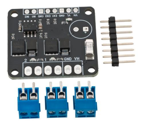
EKM013 and EKM014 are two small modules with two (EKM013) and four (EKM014) powerful FETs for driving heavy loads. The FETs are controlled by a very fast driver IC from Ti that can toggle the transistors fully on and off at extremely high frequencies.
