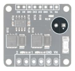
The board has space for a large electrolytic capacitor that can be installed if necessary. The capacitor is normally not required for small loads and is not included. The pattern will fit capacitors with 3.5mm pitch and a diameter of 8mm (max 10mm). Be observant of the capacitor voltage rating! The working voltage should be higher than FET voltage supply with some margin and the capacitor should be a low impedance model.
