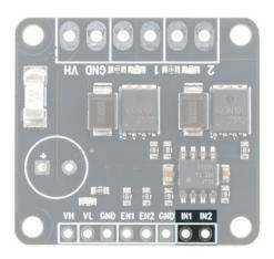
The logic supply voltage and control inputs are all arranged on one side of the board. The connector pitch is 2.54mm and will fit any standard pin header.
