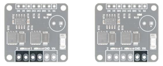
The connections for the two channels and FET voltage supply are made using 3.5mm pitch screw terminals (or by soldering wires directly to the board).
