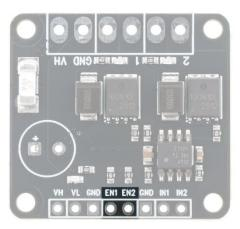
The 2-channel board EK013 breaks out the enable inputs from the driver IC to enable external control of the two inputs. The enable pins are pulled high and can be left floating if unused. Pull to GND to disable the channel.
