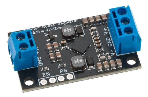
Power supply module based around a dual output switching voltage regulator, to provide a bipolar output voltage of -12V and +12V. Very useful for powering OP-amplfifiers, ADCs, DACs, and other analog circuits that require both positive and negative voltages.
