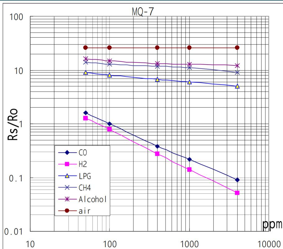
This shows the typical sensitivity characteristics of the MQ-7. Rs means resistance of the sensor in different gases, Ro means resistance of sensor in
