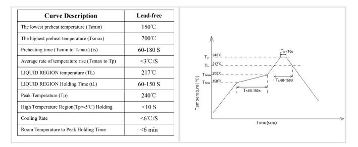
Remarks: 1. These general guidelines may not apply to all PCB designs and reflow soldering configurations.
