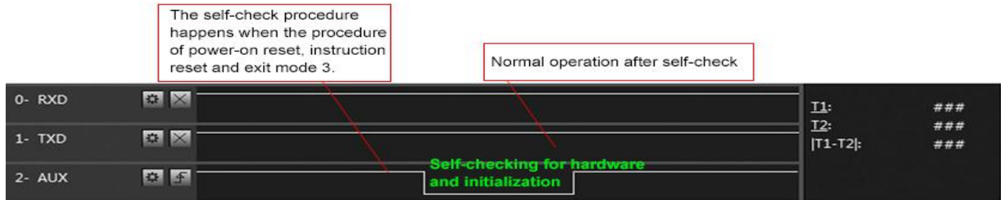
Timing Sequence Diagram of AUX when self-check
