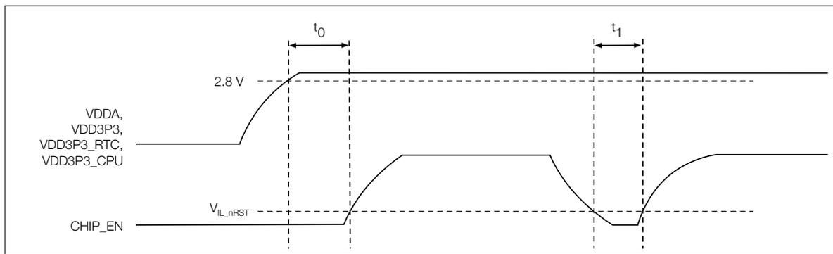
Figure 5: ESP32-C3 Family Power-up and Reset Timing
