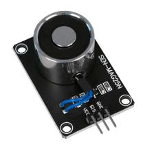
This electromagnet is suitable for smaller projects (e.g. in automation, microcontrollers or robotics). At 5 V, it generates a force of approx. 25 N (approx. 2.5 kg).
