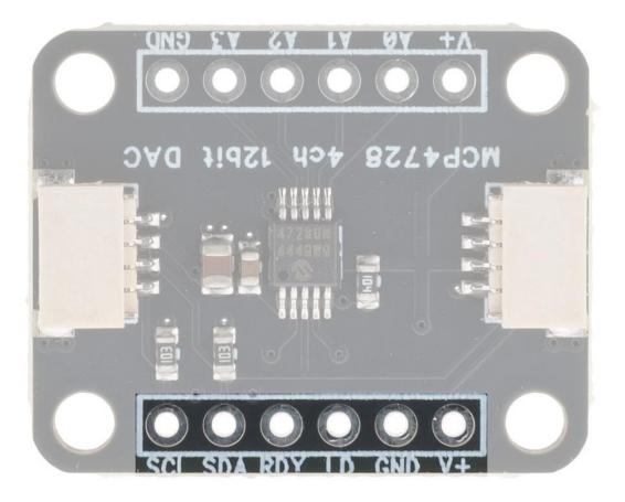
Connect V+ and GND to a voltage supply between 2.7V and 5.5V.
