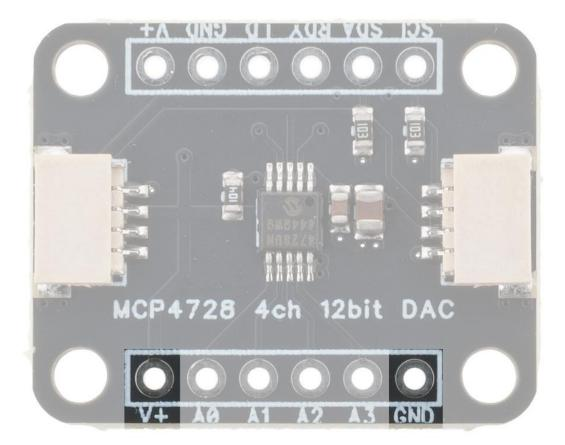
V+ and GND on this side of the board are connected to the same nets as V+ and GND on the other side and can be used to supply other modules and components, like OP- amps, filters or bias resistors.
