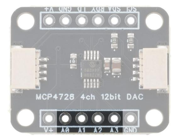
The four voltage outputs from the DAC are aligned along one side of the board. The outputs are ground referenced and have limited drive capability, around 20mA per pin. The output impedance is 1 ohm. When the chip is powered down, the output buffers are disconnected from the DAC and can be set to a known resistance of 1k, 100k or 500k, to ground.
