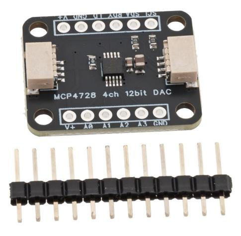
DAC module based around Microchip MCP4728, 4-channel 12-bit DA-converter. The onboard EEPROM can store configuration and DAC codes to make it start with the last DAC values after power-down. This is useful for applications where the DAC is used for calibration and the voltage only needs to be set once or infrequently.
