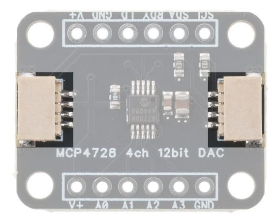
Two QWIIC connectors are available for fast and easy wiring using QWIIC cables. The QWIIC system contains V+, GND, SCL and SDA signals. LDAC and RDY/BSY must be wired separately.
