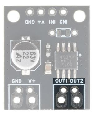
The motor outputs have dual patterns for either 2.54mm headers or 3.5mm screw terminals (included).
