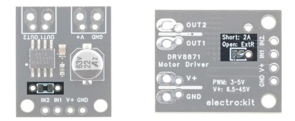
DRV8871 features a simple current limiting using just one resistor. The breakout board comes with a resistor pre-installed for a limit of 2A. The default current limit is usually enough to drive most small motors. It can be changed to allow the full 3.5A the driver is capable of, or to limit the current further to protect very small motors.
