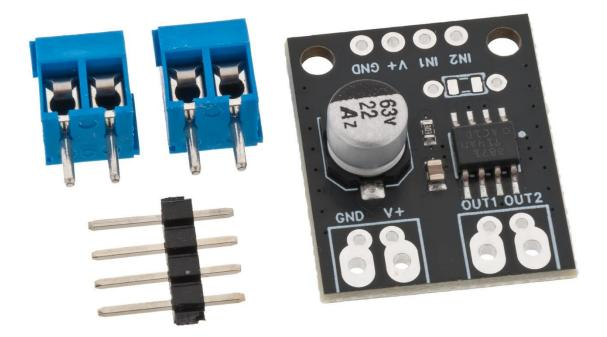
Small breakout board for Texas Instruments DRV8871 Single channel DC motor driver. The driver is controlled with two PWM signals and will drive a connected DC motor in both directions. The inputs will accept both a static DC voltage to run the motor at 100% or PWM signals to vary the speed. When both inputs are low, the motor is disconnected from the driver outputs and is free to spin (coast). When both inputs are high, the motor will be braked and resist rotation.
