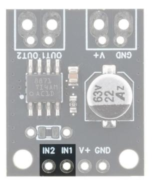
Using DRV8871 is very simple and requires just two control pins to make the motor go forward, backward, break or coast.
