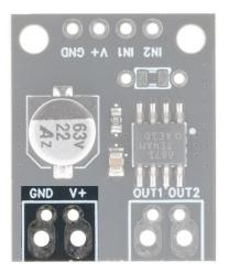
The supply voltage range is 6.5 - 45 VDC and should be connected to EITHER the pins adjacent to IN2/IN1 OR via the screw terminals on the output side of the board. Please note that the GND pins must be connected to both the microcontroller and external power supply to establish a common ground for the driver and logic signals.
