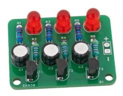
transistor in the oscillator. The kit is suitable as a first solder practice or as a demonstration of transistors, self-amplification and oscillators.
