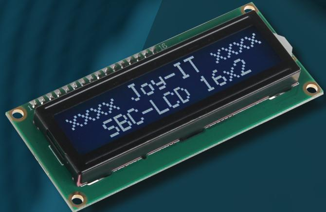
The SBC-LCD16x2 is a compact 2.6“ LCD module with 2 lines of 16 characters each and is ideal for embedded applications, control systems, prototyping and DIY electronics projects. The integrated blue backlight ensures good readability even in difficult lighting conditions.
