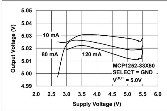
**FIGURE 2-1:** Output Voltage vs. Supply Voltage (MCP1252-33X50).
