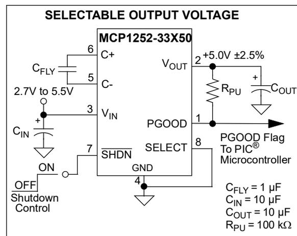
FIGURE 5-1: Typical Circuit Configuration for Fixed Output Device.
