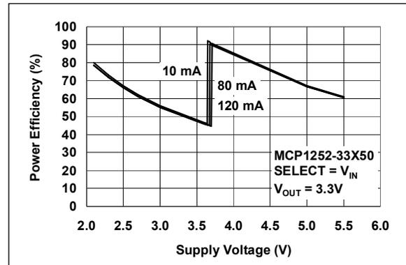
**FIGURE 2-5:** Power Efficiency vs. Supply Voltage (MCP1252-33X50).
