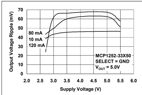
**FIGURE 2-13:** Output Voltage Ripple vs. Supply Voltage (MCP1252-33X50).
