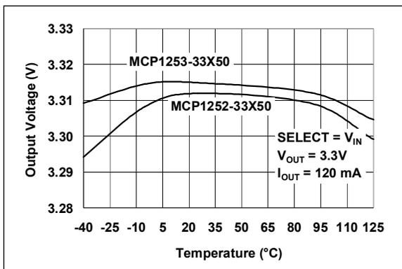
**FIGURE 2-8:** Output Voltage vs. Temperature (MCP1252-33X50, MCP1253-33X50).
