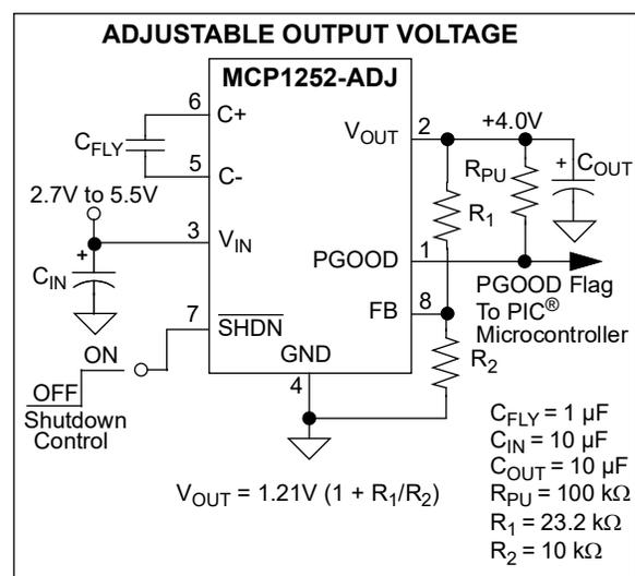
FIGURE 5-2: Typical Circuit Configuration for Adjustable Output Device.
