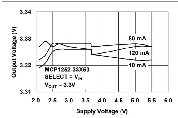
**FIGURE 2-2:** Output Voltage vs. Supply Voltage (MCP1252-33X50).
