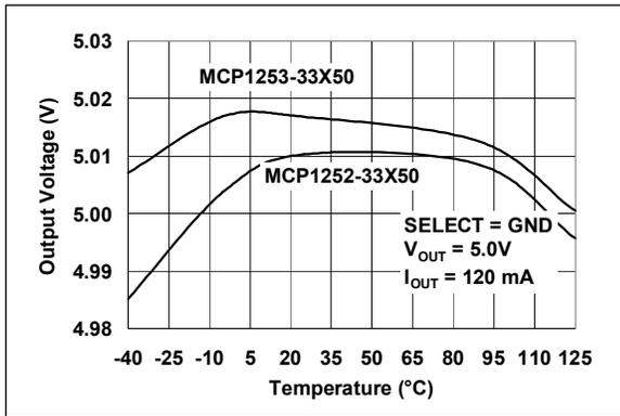
**FIGURE 2-7:** Output Voltage vs. Temperature (MCP1252-33X50, MCP1253-33X50).
