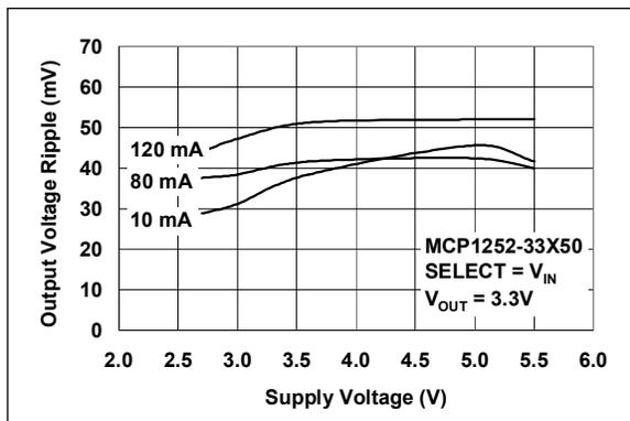
**FIGURE 2-14:** Output Voltage Ripple vs. Supply Voltage (MCP1252-33X50).
