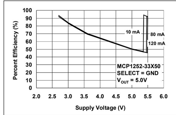
**FIGURE 2-4:** Percent Efficiency vs. Supply Voltage (MCP1252-33X50).
