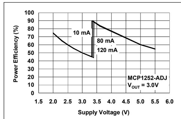
**FIGURE 2-6:** Power Efficiency vs. Supply Voltage (MCP1252-ADJ).
