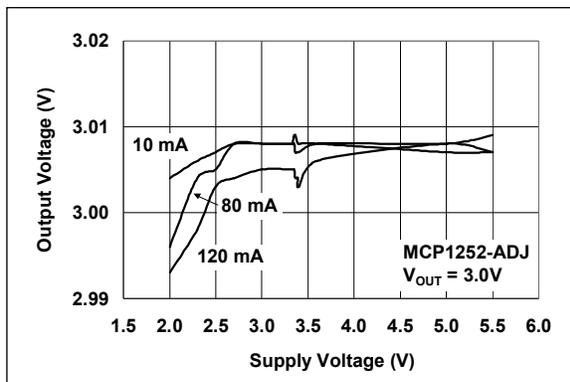
**FIGURE 2-3:** Output Voltage vs. Supply Voltage (MCP1252-ADJ).
