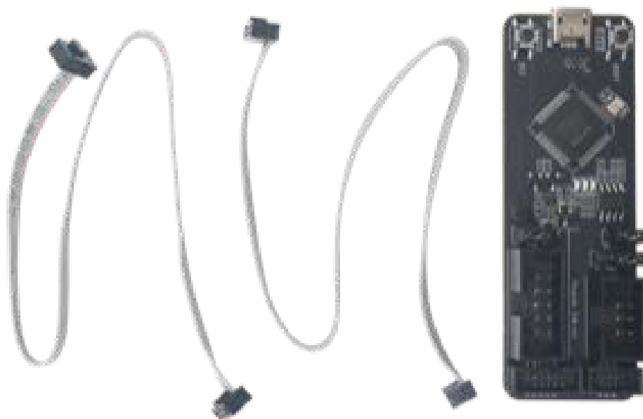
Fig. 3: ESP-Prog Package Contents
