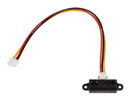
This infrared distance sensor can measure distances up to 80cm fast and reliably. The reaction time is about 39 milliseconds.
