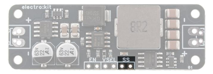
If the connected load has a large amount of capacitance, the inrush current can be limited by soft-starting the regulator. By default, the module is configured for a 5ms ramp-up, which is appropriate for most applications. If a longer ramp-up is required, a capacitor can be connected between the SS pins. The capacitor can be calculated using the formula in the LMR14050 datasheet on page 18.
