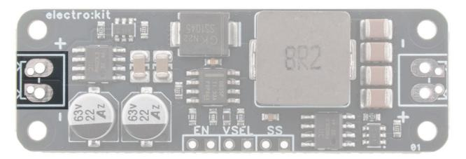
The module can be supplied with a DC voltage between 4 and 40V, but must be 1V higher than the selected output. For 3.3V output, VIN must be ~4.5V and for 5V out, ~6V.
