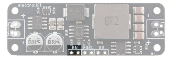
The enable input can be used to put the regulator to sleep and reduce the quincent current to 1µA.
