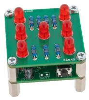
The kit is delivered as two circuit boards that are linked together with four copper traces. For a somewhat simpler assembly process, you can just solder the components in place and leave the boards connected. Solder wires to V+ and GND, and the die is ready to use.
