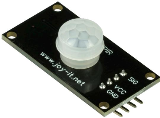
The SBC-PIR is a powerful PIR motion sensor that has been specially developed for use in embedded systems, single-board computers and microcontroller projects. The sensor reliably detects movements in a detection range of around 120 degrees and provides a clean, digital output signal that can be analysed directly by common systems such as Raspberry Pi, Arduino or ESP32.
