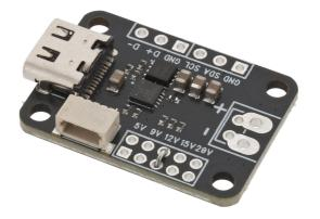
Before use, the module must be configured to request the desired voltage from a connected USB power supply. A  $2\times5$ -pin header is included in the package and can be soldered to the board for a quick and easy way to change the voltage using the included jumper. For a more permanent and low-profile application, a simple wire or component lead can be used instead of the entire pin header.
