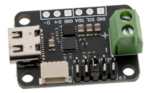
This module, when connected to a PD (Power Delivery) enabled USB power supply, will negotiate with the power supply to output a selectable voltage from 5V up to 20V. To configure the output voltage, simply place the jumper on the corresponding pins. Since the PD controller is configurable via I2C, these pins are also exposed for advanced users.
