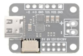
To configure the PD controller and change the output voltage and current limit from a microcontroller, I2C pins are broken out both as individual pins and as a JST-SH 1.0mm QWIIC connector. The PD controller works as an I2C slave on address 0×08. I2C takes priority over the manual voltage setting. External pullup resistors for SCL/SDA must be used.
