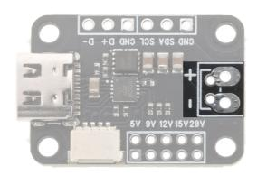
The voltage from the USB power supply is provided on the large pads opposite the USB connector. Please be observant of the polarity markings! The pads will fit either a 2.54mm pitch connector (screw terminal or pin header) or the included 3.5mm pitch screw terminal. Wires can also be soldered directly to the board for space-constrained applications.
