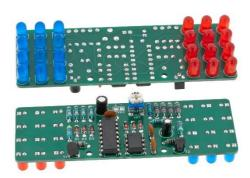
the driving capability of the decade counter, the LEDs are connected via individual NPN transistors, each capable of sinking up to 200mA of current per color..
