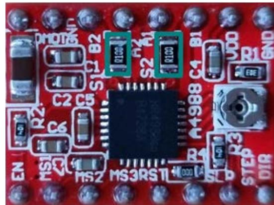
**$V_{\text{REF}}$  (reference voltage)** is the value that must be set on the rotary potentiometer.
