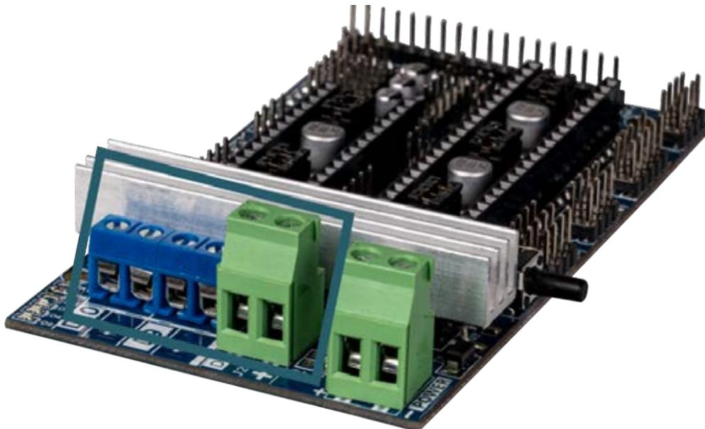
Finally, the expansion board must now be supplied with power. Please note that your expansion board has two connectors. One for 11 amps and one for 5 amps. Both connections can be supplied with a maximum of 12 V.
