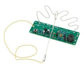
a tone in the speaker as soon as the copper wire is touched with the loop. The game is reset with the push button on the circuit board.
