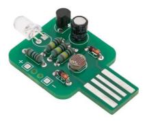
connector, which provides a simple way to both mount and power the kit. It can be plugged into a USB port of a computer or a USB charger. The two diodes makes it possible to insert the board either way into a USB port. Two holes marked "+" and "-" can be used as an alternate input from any regular DC power source. To change the sensitivity, mount either one, two or all three 1 Mohm resistors. One resistor provides high sensitivity, two medium and with all three mounted, lowest sensitivity.
