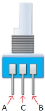
A rotary encoder has a fixed number of positions per revolution. These positions are easily felt as small “clicks” you turn the encoder. On one side of the switch there are three pins. They are normally referred to as A, B and C.
