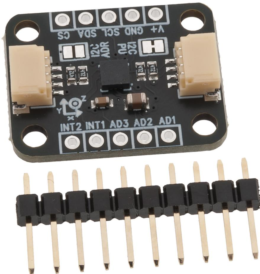
Breakout board with QWIIC connectors for the low-power 3-axis accelerometer from ST. The accelerometer has high resolution outputs for three spatial axis (x, y, z), temperature and also three (ADC3 is shared with internal temperature sensor) additional ADC channels that can be used for connecting external, analog sensors and digitize their outputs together with the internal outputs from the accelerometer.
