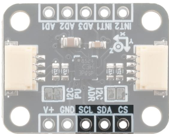
SCL, SDA and CS are all pulled high using 4.7k resistors. Pullups for SCL and SDA can be disabled by severing the I2C PU solder jumper.
