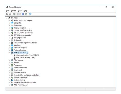
Sometimes the item will refer to the name of the board. Other times it may be called something like USB Serial Device, as seen in the image above. Either way, there is a new (COM#) following the name. This is the port your board is using.
