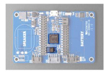
The main processor chip is the ATSAMD51J19 Cortex M4 running at 120MHz with 3.3v logic/power. It has 512KB of Flash and 192KB of RAM. We also include 2 MB of QSPI Flash for storing images, sounds, animations, whatever!
