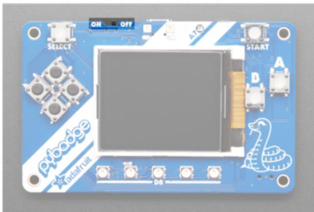
On/Off switch - Powers off the board. Even if plugged in, the board won't work if switched to off. You can charge the battery when the board is off, but the USB device will not be active or any other electronics
