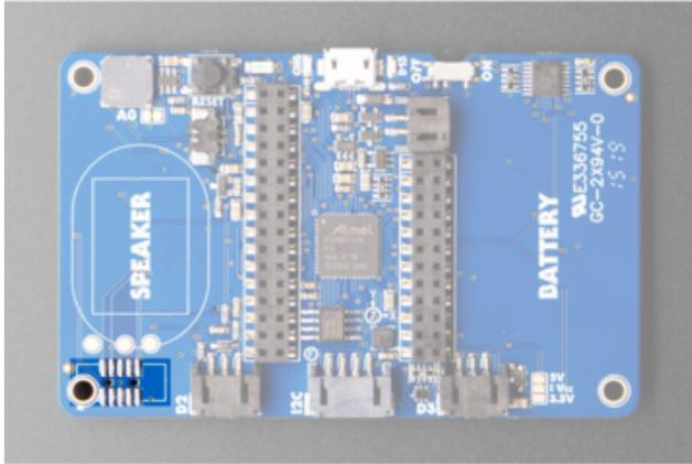
The unpopulated 10 pin footprint located in the bottom left corner is for an SWD connector. It is meant for use with a connector like [this \(\)](#) or [this \(\)](#). Once wired up, you can use it for debugging with a JTAG debugger.
