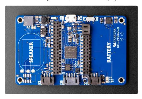
The back features various connections for add-ons, space for a speaker and a battery, a tiny built-in speaker, an accelerometer and more. Let's take a look!
