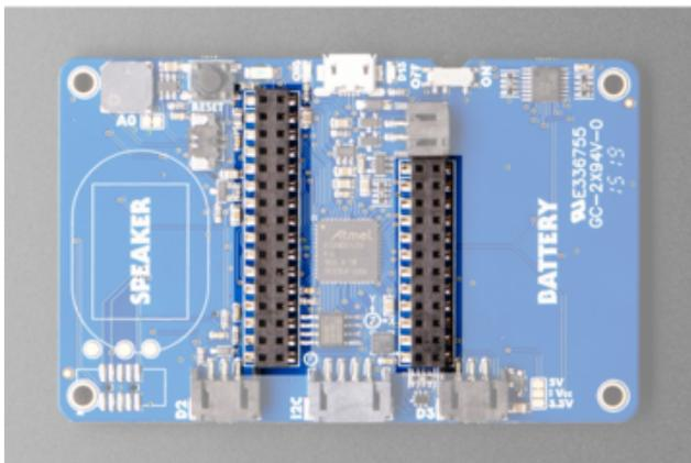
You can easily attach FeatherWings to the back of your PyBadge using the convenient "Feather Headers" on the back. Located in the middle, they break out all the same pins you have access to on a Feather board, allowing use of any of our wide range of FeatherWings. Easily add all kinds of functionality to your PyBadge! The GPIO is all 3.3V logic.
