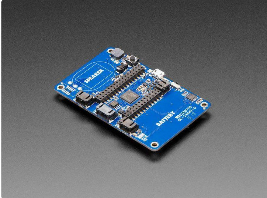
On the back of the PyBadge we have a full Feather-compatible header socket set, so you can plug in any FeatherWing to expand the capabilities of the PyBadge. There's also 3 STEMMA connectors - two 3-pin with ADC/PWM capability and one 4-pin that connects to I2C - you can use this for Grove sensors as well. The PyBadge LC does not include the feather header or STEMMA connectors, to make it lower cost
