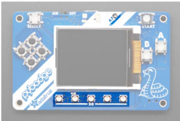
Light sensor (A7) - There is an ambient light sensor on the top, which points through to the front. The light sensor is an analog input, connected to `board.LIGHT` (CircuitPython) or `A7` (Arduino) you can read it as any analog value ranging from 0 (dark) to 1023 (in Arduino) or 65535 (CircuitPython) when bright.
