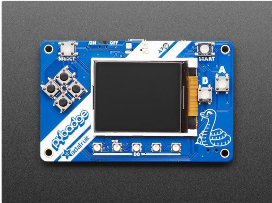
What's the size of a credit card and can run CircuitPython, MakeCode Arcade or Arduino? That's right, it's the Adafruit PyBadge and little sister Adafruit PyBadge LC! We wanted to see how much we could cram into a  $3 \frac{3}{8} \times 2 \frac{1}{8}$  inch rounded rectangle, to make an all-in-one dev board with a lot of possibilities, and this is what we came up with.
