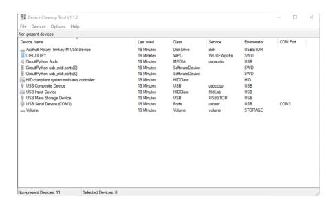
Select all the devices you want to remove, and then press Delete. It is usually safe just to select everything. Any device that is removed will get a fresh install when you plug it in. Using the Device Cleanup Tool also discards all the COM port assignments for the unplugged boards. If you have used many Arduino and CircuitPython boards, you have probably seen higher and higher COM port numbers used, seemingly without end. This will fix that problem.
