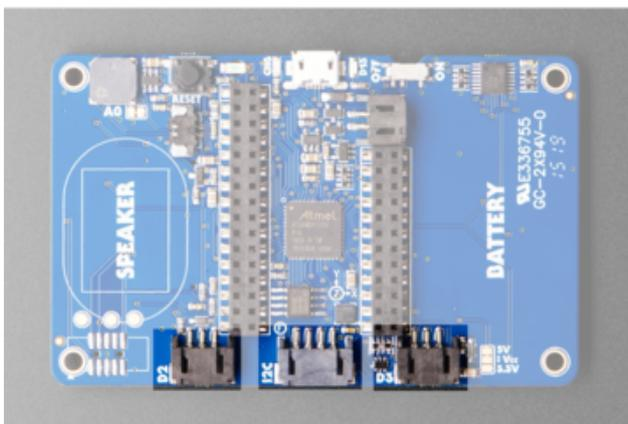
There is a 4-pin JST I2C connector in the center on the bottom, that is STEMMA and Grove compatible. You can access VCC power and ground as well as a level-shifted `SDA` & `SCL` connection. In CircuitPython, you can use the STEMMA connector
