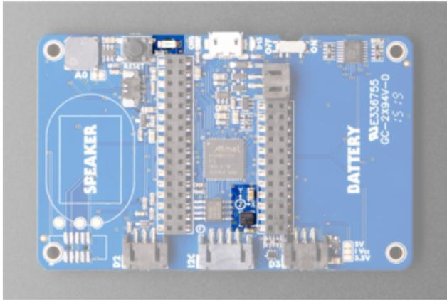
Accelerometer - The PyBadge has an accelerometer located near the middle, above the I2C connector. It is an LIS3DH. The PyBadge LC does not include an accelerometer
