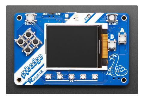
Adafruit PyBadge is the size of a credit card, but it's loaded with all kinda of goodies. The front has buttons, LEDs, a light sensor, and a built-in display.
