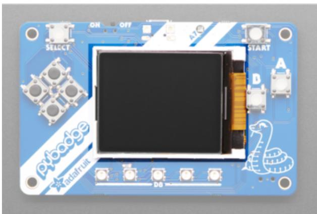
1.8" TFT display - The front features a 160x128 pixel color display.
