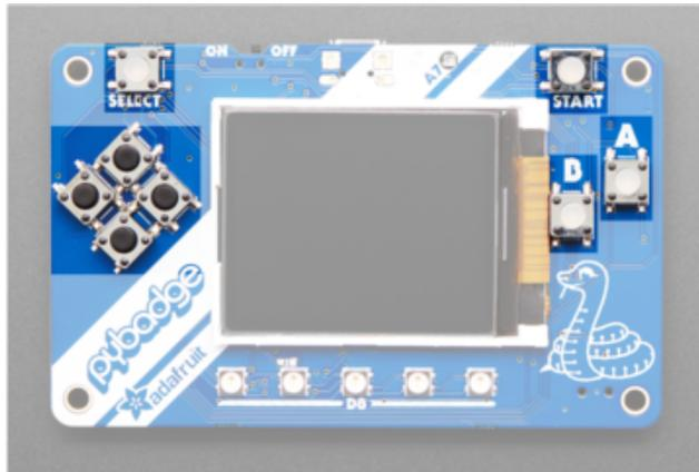
Buttons - There are 8 buttons on the front: A, B, Select, Start and four arranged in a d-pad. These buttons do not connect to GPIO pins directly. Instead they connect to an 8-channel shift register to save pins. This doesn't matter to you as long as you use the Arduino/MakeCode/CircuitPython functions to read the button presses
