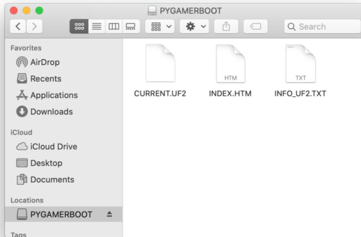
The bootloader version is listed in **INFO\_UF2.TXT**. In this example, the version is V3.6.0.
