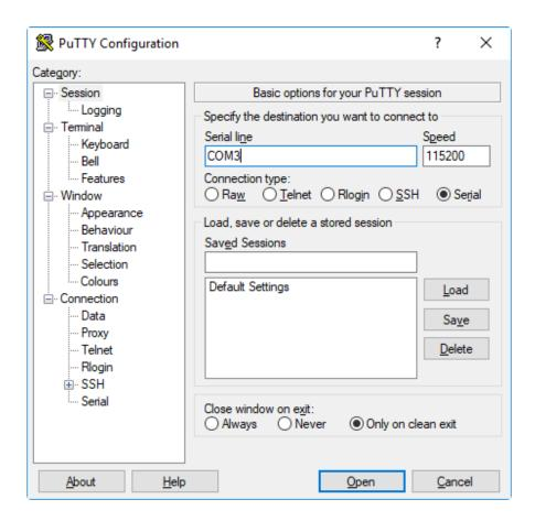
Once your settings are entered, you're ready to connect to the serial console. Click "Open" at the bottom of the window. A new window will open.
