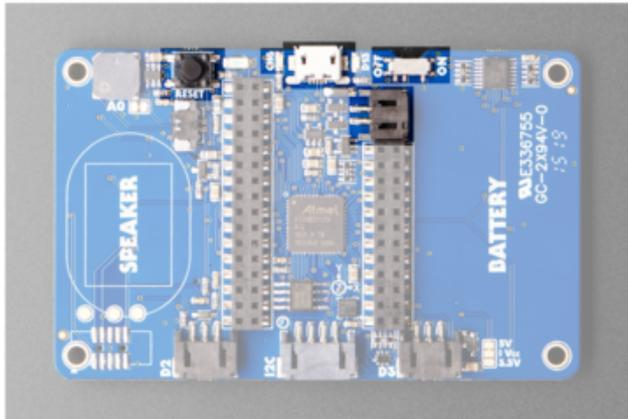
The On/Off switch is located on the top. There is one USB port on the board. On the left side, towards the bottom, is a USB Micro port, which is used for powering and programming the board.
