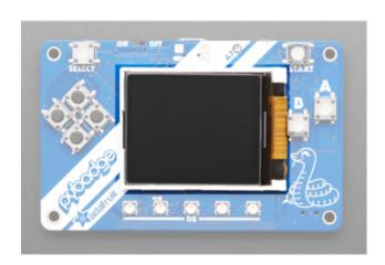
1.8" TFT display - The front features a 160x128 pixel color display.
