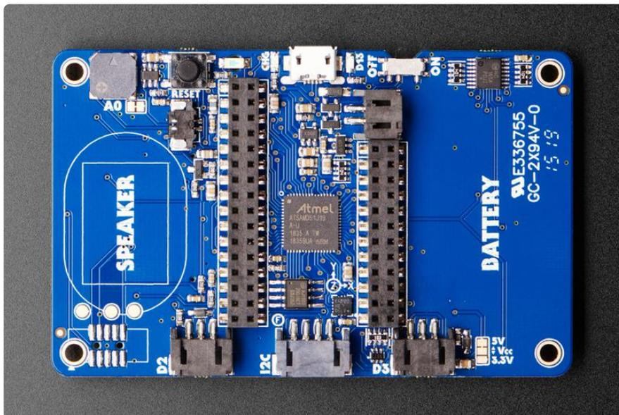
The back features various connections for add-ons, space for a speaker and a battery, a tiny built-in speaker, an accelerometer and more. Let's take a look!
