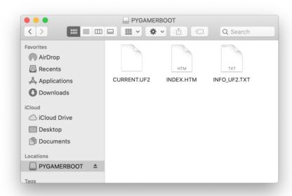
The bootloader version is listed in <a href="INFO\_UF2.TXT">INFO\_UF2.TXT</a>. In this example, the version is V3. 6.0.
