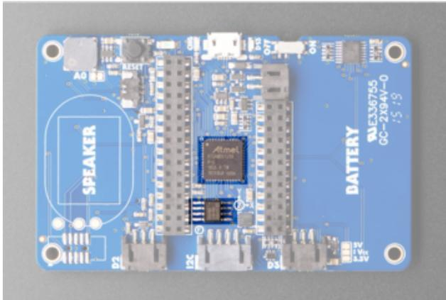
The main processor chip is the ATSAM51J19 Cortex M4 running at 120MHz with 3.3v logic/power. It has 512KB of Flash and 192KB of RAM. We also include 2 MB of QSPI Flash for storing images, sounds, animations, whatever!
