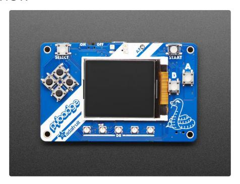
What's the size of a credit card and can run CircuitPython, MakeCode Arcade or Arduino? That's right, its the Adafruit PyBadge and little sister Adafruit PyBadge LC! We wanted to see how much we could cram into a  $3.3/8 \times 2.1/8$  inch rounded rectangle, to make an all-in-one dev board with a lot of possibilities, and this is what we came up with.
