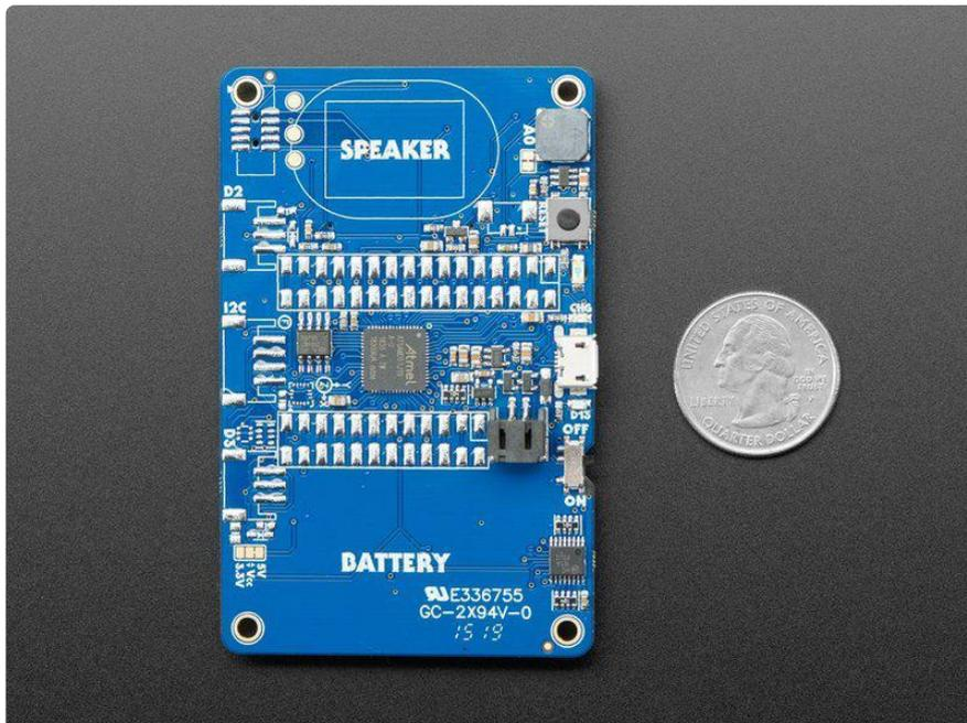
For built in sensors, there's a light sensor that points out the front, and the PyBadge has a 3-axis accelerometer that can detect taps and free-fall. To make bleeps and bloops, there's a built in buzzer-speaker. [For projects where you need more volume, you can plug in one of our 8 ohm speakers \(\)](#) on the PyBadge. (The LC does not come with accelerometer or speaker plug, but it does have a buzzer and light sensor)
