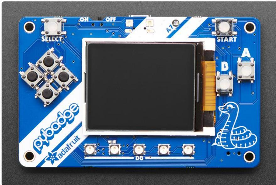
Adafruit PyBadge is the size of a credit card, but it's loaded with all kinds of goodies. The front has buttons, LEDs, a light sensor, and a built-in display.
