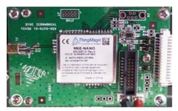
The Nano Carrier Board is an example of a host board to create an assembly that is compatible with the standard Development Kit main board. It has the size and dimensions of the M6e module (69 mm x 43 mm) and uses the same connector for power and control (Molex 532611571 - 1.25mm pin centers, 1 amp per pin rating, which mates with Molex housing p/n 51021-1500 with crimps p/n 63811-0300).
