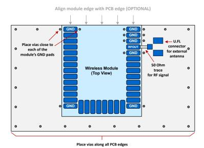
Figure 7.2. Recommended Layout for MGM240P Using External Antenna
