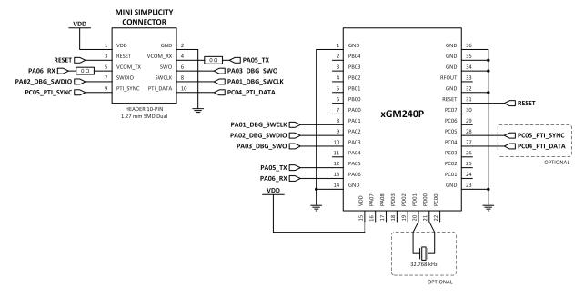
Figure 5.2. Stand-Alone SoC Configuration
