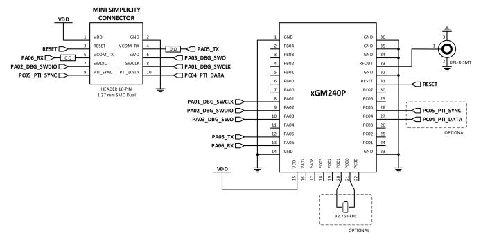
Figure 5.3. Stand-Alone SoC Configuration with External Antenna
