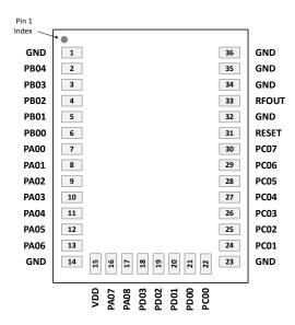
Figure 6.1. MGM240P Module Pinout
