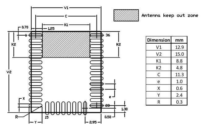
Figure 8.3. Recommended Land Pattern for Modules with a Built-in Antenna
