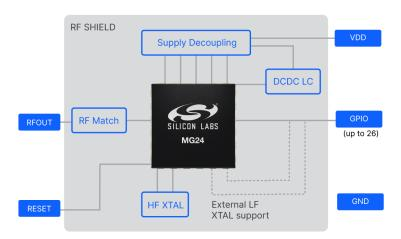
Figure 3.2. MGM240P Block Diagram - RF pin Variant
