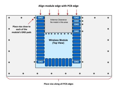
Figure 7.1. Recommended Layout for MGM240P Using Built-in Antenna
