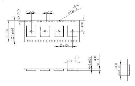
Figure 10.1. Carrier Tape Dimensions
