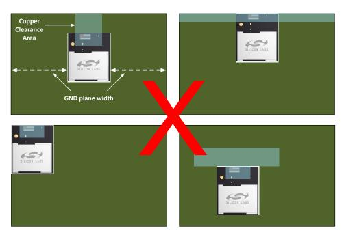
Figure 7.3. Non-Optimal Layout Examples
