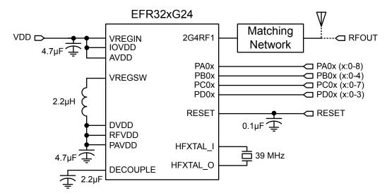
Figure 3.3. MGM240P Module Schematic
