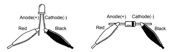
The Anode(+) of the LED or diode should be connected to the red probe. The Cathode(-) of the LED or diode should be connected to the black probe.
