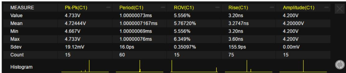
Touch the histogram area of a parameter to enlarge it for details. You can move the large histogram window position around the display by dragging. Touch the histogram of another parameter to switch to the corresponding enlarged histogram.
