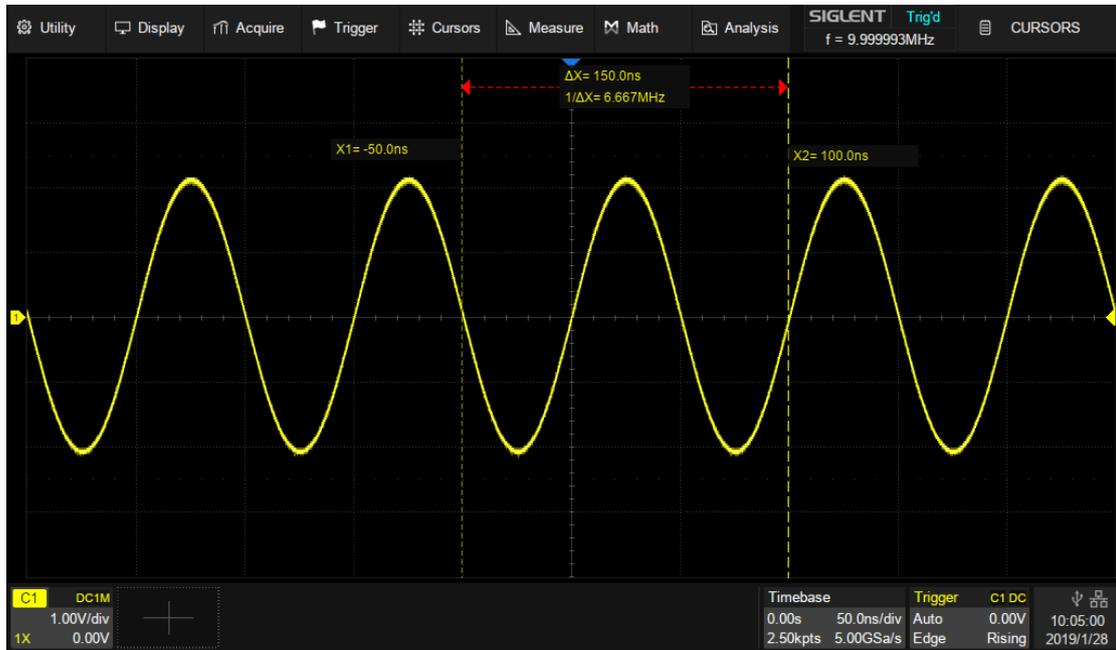
Timebase=50ns/div,  $X1 = -50\text{ns} = -1\text{div}$ ,  $X2 = 100\text{ns} = 2\text{div}$
