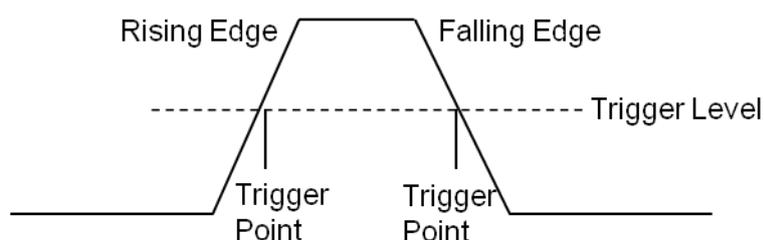
Touch the **Source** area to select trigger source, and touch the **Slope** area to select rising, falling or alter.
