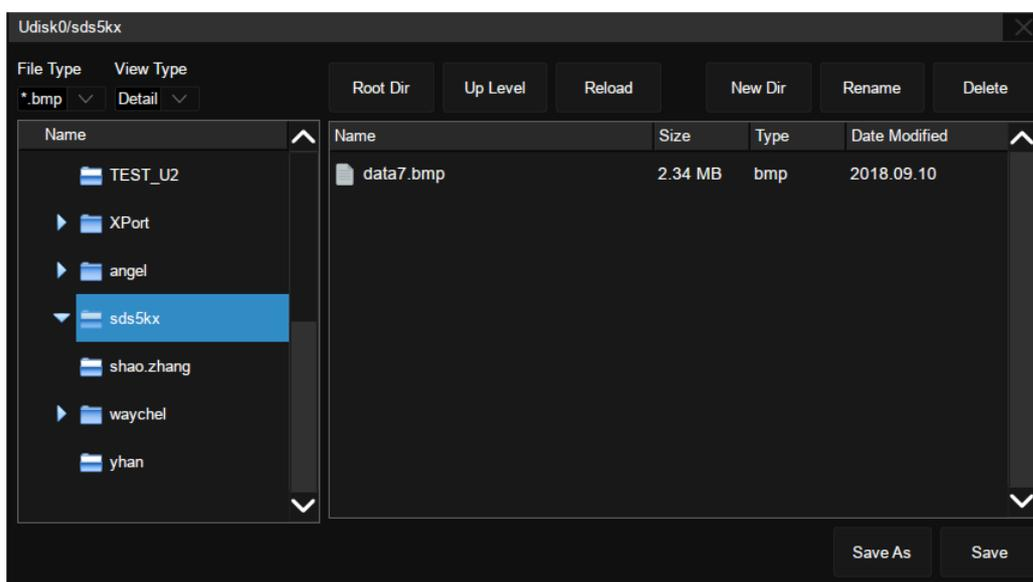
In step 4, if **Save** is selected instead of **Save As**, the system saves the file as the default file name sds5000x\_n.bmp, where n is an integer incrementing from 1. The default save path is \SIGLENT\.
