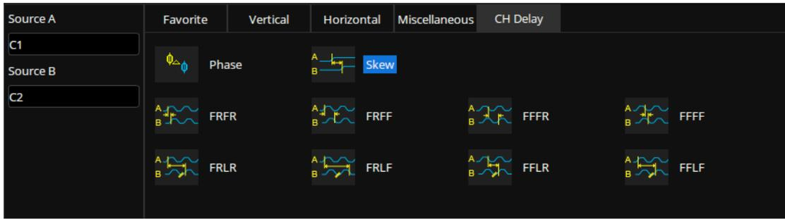
In the parameter selection area, the channel corresponding to **Source A** is specified first, and then the channel corresponding to **Source B**. Finally, the measurement parameter is selected. For example, to activate the skew between C1 and C2, you can follow the following steps:
