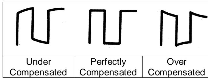
5. Use a non-metallic driver to adjust the low-frequency compensation adjustment hole on the probe until the waveform displayed is as the “Perfectly compensated” in the figure above.
