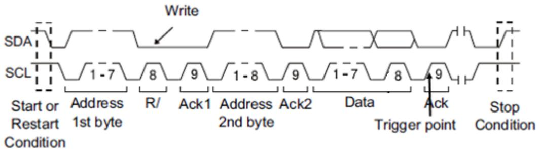
If you set the trigger condition to 7 address & data or 10 address & data:
