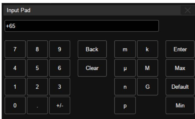
Let's use the operation of setting the "deskew" of a channel as an example: If the expected value is 65 ns, input "65" on the virtual keypad, and then choose the unit **n** to complete the operation. On the virtual keypad, touching the button **Max**, **Min**, and **Default** quickly sets the parameter to its maximum, minimum and default values.
