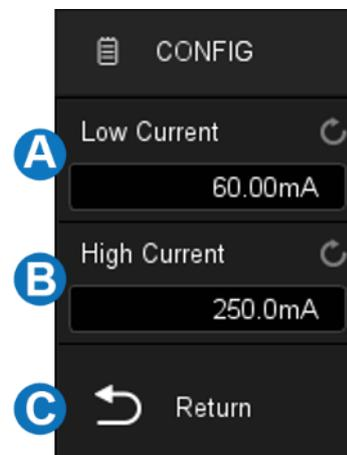
**Note:** low current value and high current value are used to calculate trigger level and adjust the oscilloscope vertical scale. After the load changes, the current value changes from low to high (or from high to low), and the oscilloscope triggers and performs to measure the transient response stability time.
