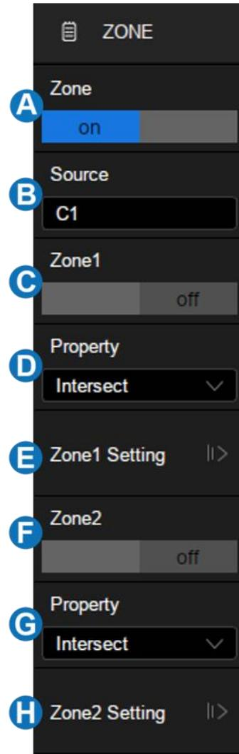
The zones can be created and moved by gestures or by setting **Zone> Zone Setting** in the dialog box. The color of the zone’s outline is consistent with the color of the specified source (Channel 1 = Yellow, etc...).
