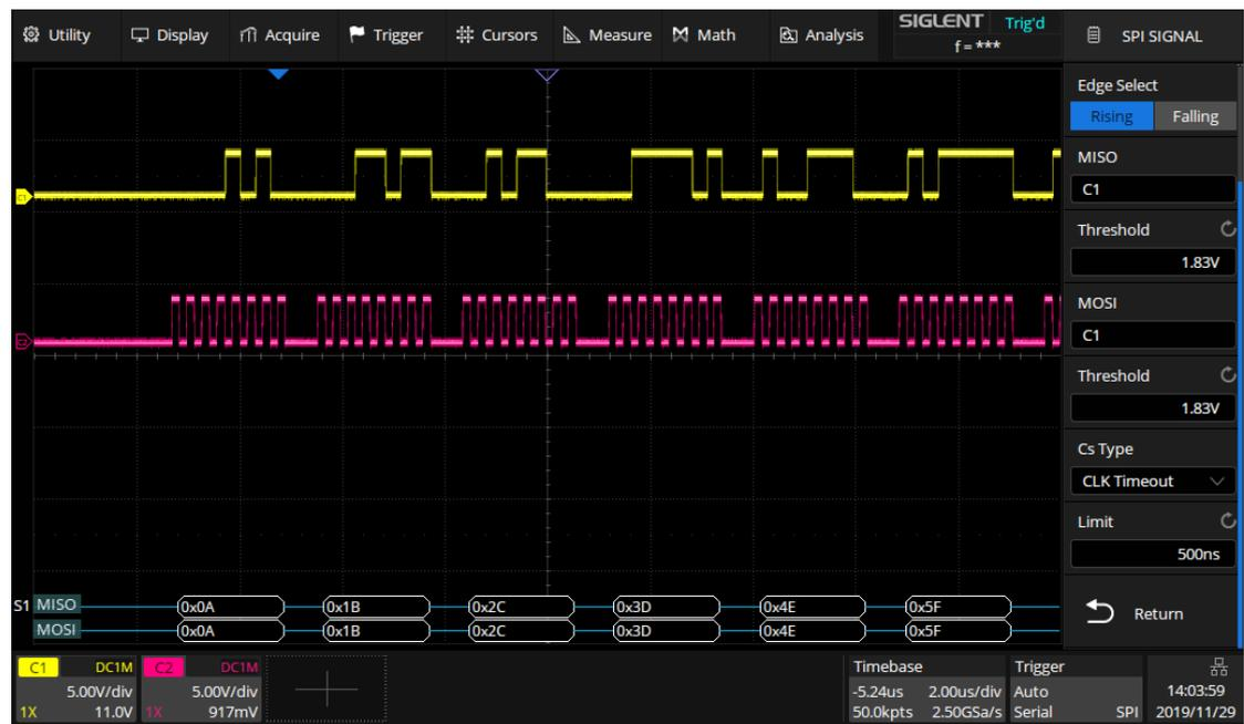
If the data width is set to be greater than 8 bits (such as 16 bits), measure the clock idle time between 8-bit data packets as 0.57 us, and then set the timeout time to a value between 0.57 and 150 us. In this example, it is set to 1 us:
