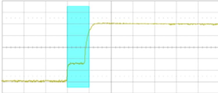
With a simple edge trigger, it is unlikely to trigger consistently on this anomaly. Thanks to the high waveform update rate of the SDS5000X, we can confirm there is bus contention happening by enabling the persistence display, as shown in the figure below:
