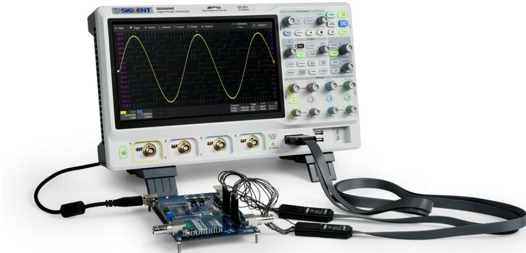
**To connect the logic probe:** Insert the probe, with the correct side facing up, until you hear a “click”.
