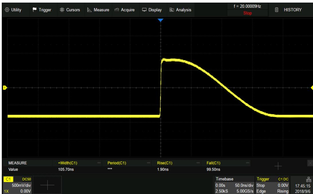
In the example, 53969 pulses can be obtained with the sample rate of 5 GSa/s at the maximum memory depth.
