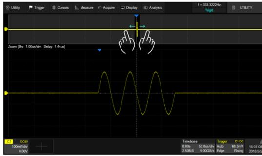
Adjust the horizontal scale of main window by pinch and spread in the gray area of the main window
