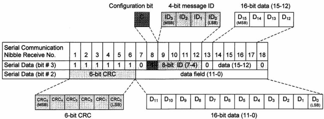
Frame (enhanced serial message with 8bits ID) —12-bit data and 8-bit message ID, the configuration bit is 0.
