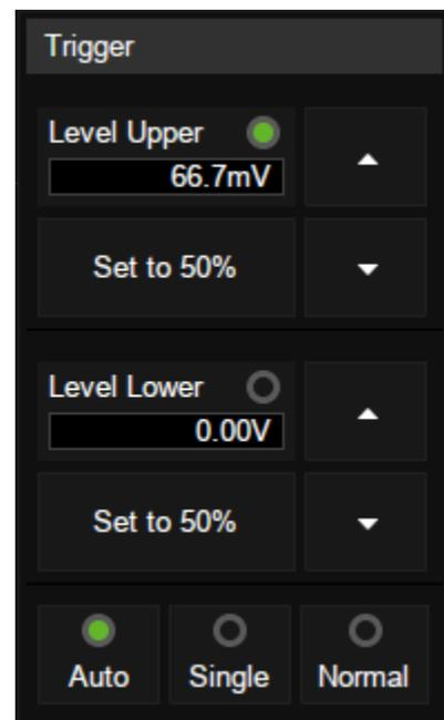
1. Touch the **Level Upper** area in the quick menu to select the upper level, and then set the level value by the virtual keypad or the **Level** knob on
