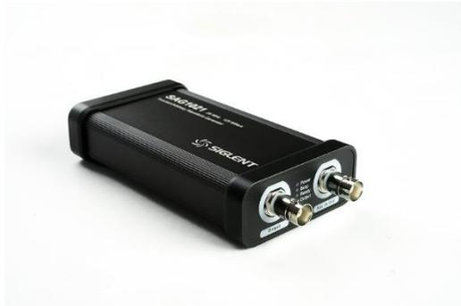
The SAG1021I function/arbitrary wave generator module is capable of generating variant waveforms with frequencies up to 25 MHz and amplitudes up to  $\pm 3$  V. Its output terminals are isolated from the ground of the oscilloscope. Users can edit and import arbitrary waveforms using the SIGLENT EasyWave software or import edited waveforms through a U-disk.
