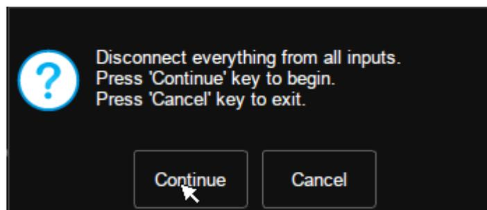
3. The oscilloscope will not response to any operate until the self-cal is finished. After the self-cal is completed, touch the screen or press any button to exit.
