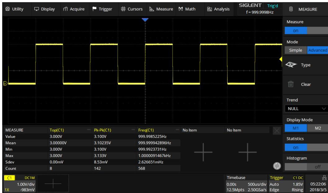
In M2 mode, up to 12 parameter measurements are displayed at a time. When statistics are enabled, they are distributed on the right side of the measurement item. Touch a row to add or replace a measurement.
