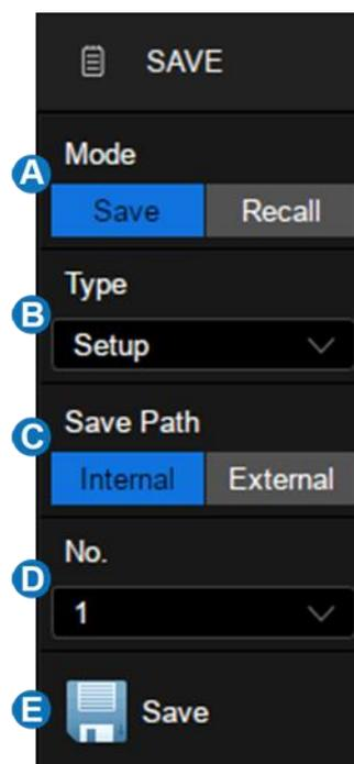
A progress bar is shown when the Save operation is in progress. When it is done, the oscilloscope prompts "Saved to internal file No.X", where X is the internal storage location index selected in the step **D**.
