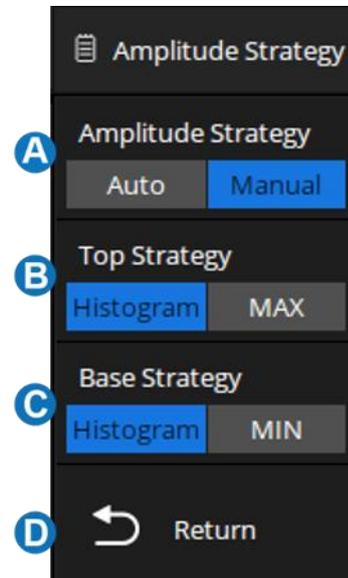
value with the maximum probability will be identified as the base value; when set to min, the minimum value of waveform will be identified as the base value
