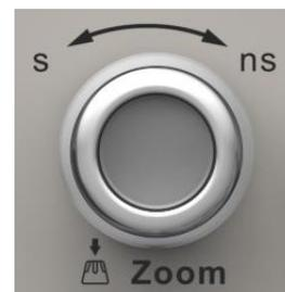
When Zoom function is on, the waveform area is divided into upper and lower parts. The area of about 1/3 height above is the main window, and the area of about 2/3 height below is the zoom window. Touch a window to activate it.
