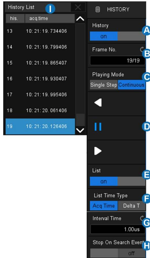
The oscilloscope automatically stores acquired frames. It can store up to 100,000 frames but the number may vary due to the memory depth and timebase settings. Turn on history mode, then the stored frames can be recalled and measured.
