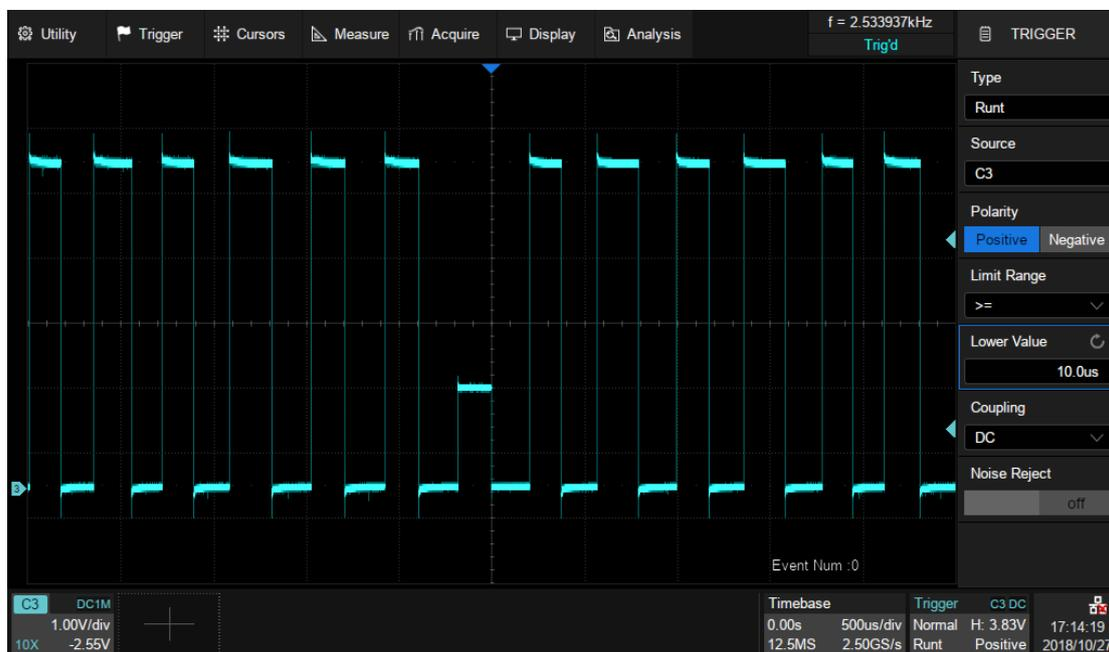
Then turn on Search function and operate *Copy from Trigger* in the search dialog box so that the oscilloscope searches for the dwarf pulses according to
