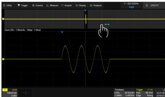
Adjust the horizontal position of the waveform by dragging left and right in the gray area of the main window
