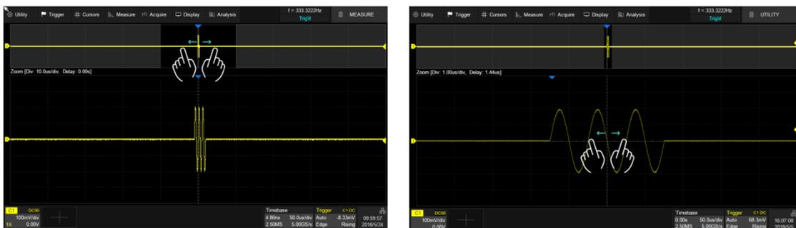
Adjust the horizontal scale of Zoom window by horizontal pinch and spread in the zoom area of the main window or in the Zoom window
