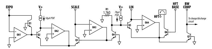
Figure 10: SSI2130 Simplified Exponential Converter
