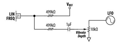
Figure 17: Linear Vibrato Keeps the Oscillator in Tune
