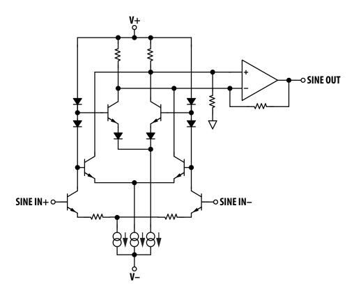
Figure 13: SSI2130 Triange-to-Sine Converter
