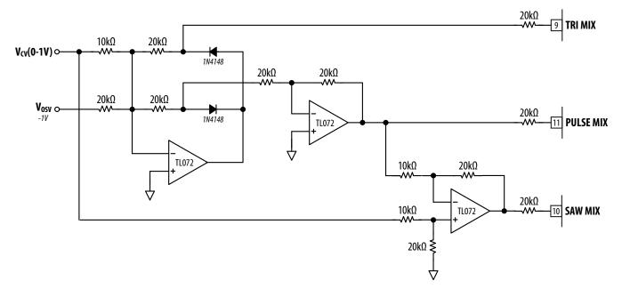
Figure 20: Triangle-Saw-PWM Cross Fader
