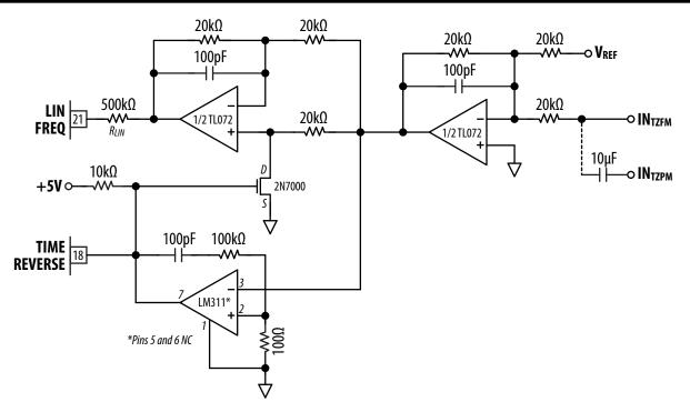
Figure 18: A Handful of Passive Makes TZFM and TZPM a Low Parts-Count Reality
