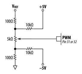
Figure 15: Ideal SSI2130 PWM Control Circuit
