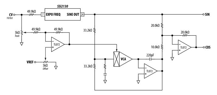
**Figure 21: A sine VCO and a tracking APF makes for Quadrature Oscillator** *Note VCA compensating component values are not shown as they depend on which variant of the SSI216x is used*
