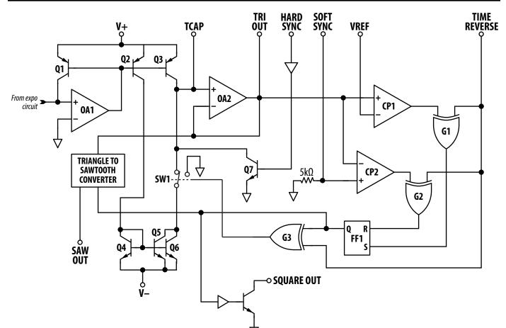
**Figure 11: SSI2130 Simplified Oscillator Core** *Triangle oscillator core can run forward or backwards depending on state of the TIME REVERSE input.*
