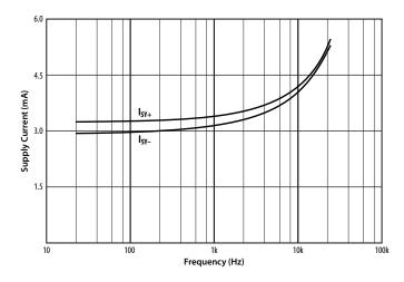
**Supply Current vs. Frequency** V+ = +5V, V- = -15V, Figure 1 Circuit
