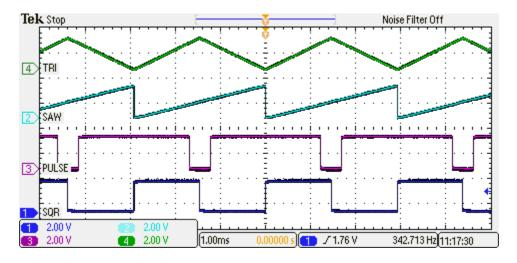
Figure 2: The SSI2130's Primary Waveforms
