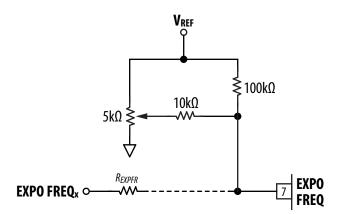
Figure 7: Expo Biasing Circuit for Manual Trim Applications
