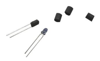
In the kit there are two rubber pads which can be used as vehicle tyres on each motors. We suggest to cut and use the smaller rubber pads as tyres, using the bigger pads will make robot faster but also not very stable.
