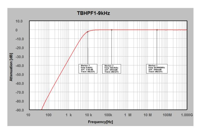
TBHPF1-9kHz: Attenuation 30 Hz to 1 GHz, typical data
