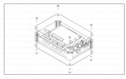
This is how your M126 LCR Meter should look once enclosure assembly is complete:
