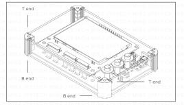
6 Assemble the top and bottom pieces with screws. Remember to attach the 3 caps to the pushbuttons before securing the top piece.
