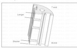
Assemble the two side pieces and back piece. Ensure the standoffs are at the correct orientation.
