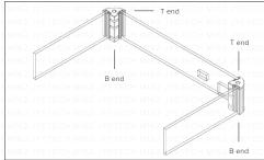
Insert the assembled main board-analog board with the analog board fitted into the standoff slots near the bottom ends.
