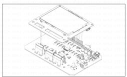
2 Apply power supply via the micro-USB connector on the analog board and slide the power switch to ON position.
