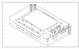
4 Assemble the front piece. Ensure the standoffs are at the corret orientation.
