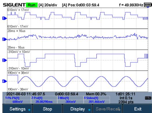
The measurement Logger is the mode of logging the measurement value for a long time. For the amount of measurement data is relatively small, to process quickly, the data is logged in memory. After stopping logging, the data can be saved into the internal flash or external U disk.
