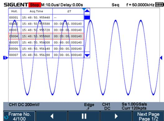
Playback the latest triggered events using the history function. Segmented memory collection will store trigger events into multiple (Up to 80,000) memory segments, each segment will store triggered waveforms and timestamps for each frame.
