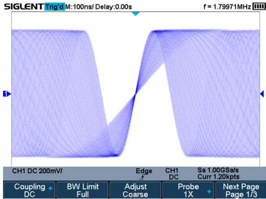
SPO display technology provides fast refresh rates. The resulting intensity-graded trace is brighter for events that occur with more frequency and dims when the events occur with less frequency.
