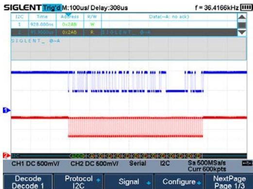
SHS800X/SHS1000X displays the decoding through the events list. Bus protocol information can be quickly and intuitively displayed in a tabular format.
