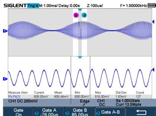
Through Gate and Zoom measurement, the user can specify an arbitrary interval of waveform data analysis and statistics. This helps avoid measurement errors that can be caused by invalid or extraneous data, greatly enhancing the measurements' validity and flexibility.
