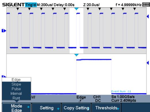
The SHS800X/SHS1000X series can search events specified by the user in a frame. It can also navigate by time (delay position) and historical frames.
