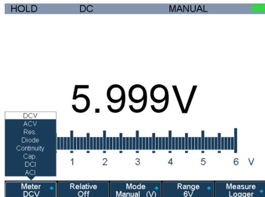
6000 count digital multimeter featured function of DCV, true RMS ACV, DCI, ACI, Diode, Resistance, Capacitance, and Continuity.
