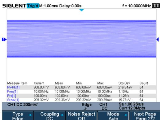
SHS800X/SHS1000X series can measure all sampled data points up to 12 Mpts. This ensures the accuracy of measurements while the math co-processor decreases measurement time and increases ease-of-use.
