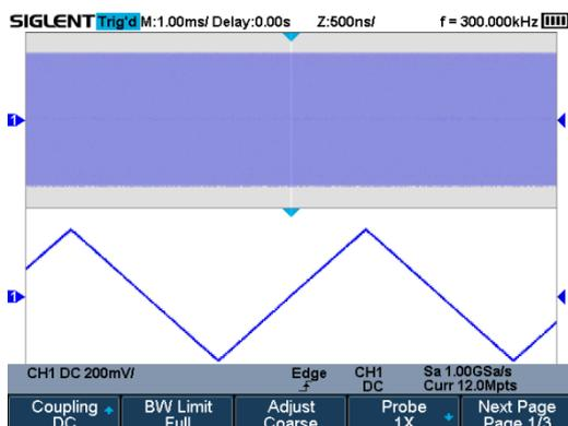
Using hardware-based Zoom technologies and max record length up to 12 Mpts, users can oversample to capture for longer periods at higher resolution and use the zoom feature to see more details within each signal.
