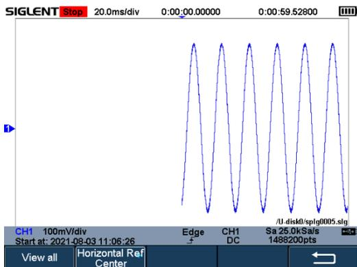
The Sample Logger is the mode of logging the sampling points for a long time. For there are many sampling points to log, they are logged into the internal flash or external U disk in real-time. After stopping logging, the user can recall the sampling points on the oscilloscope, or analyze the saved data on the computer.
