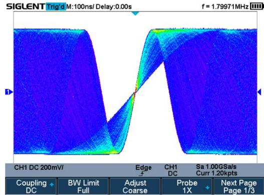
The color temperature display is similar to the intensity-graded trace function, but the trace occurrence is represented by different colors (color "temperature") as opposed to changes in the intensity of one color. Red colors represent events that occur more frequently, while blue is used to mark points that occur less frequently.
