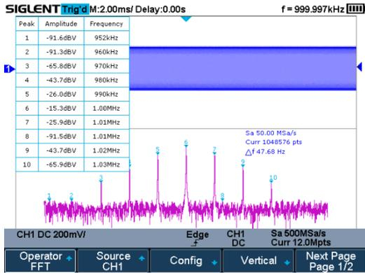
The new math co-processor enables FFT analysis of incoming signals using up to 1 M samples per waveform. This provides high-frequency resolution with a fast refresh rate. The FFT function also supports a variety of window functions so that it can adapt to different spectrum measurement needs. Support Peaks, Markers, a variety of numbers.
