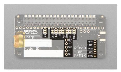
The two sets of pins here are broken out from the radio module. The defaults are:
