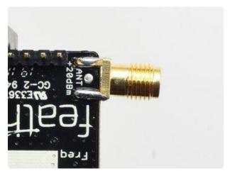
Use plenty of solder to make sure you have a good strong mechanical connection. The duck antennas are long and make great levers, so they could pry apart the solder joints if not soldered well
