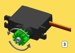
Turn the gear counterclockwise until it stops
