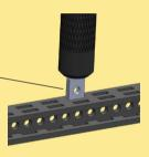
1. Use the back of the screwdriver to push in the nuts.
