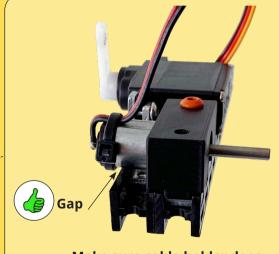
Make sure cable holder does not climb on the beam
