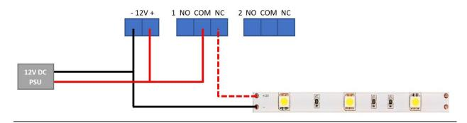
Example 2: device with different power supply voltage as the VM130V2SET with NO contacts
