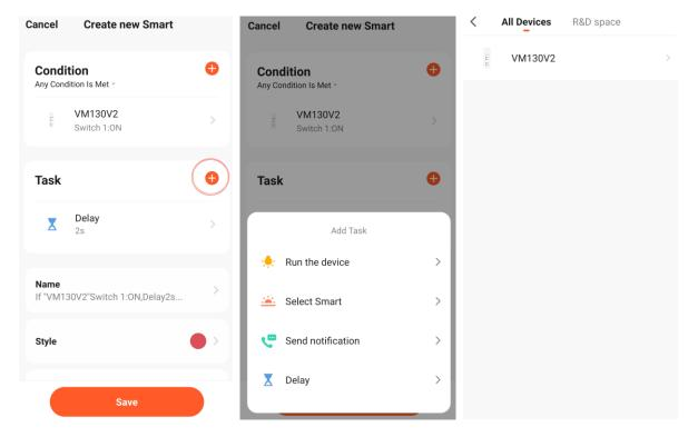
We select channel 1 (Switch 1) and the "OFF" situation. Finally, we have an overview of the set 'smart' action: When channel 1 is activated, it will switch off after a delay of 2 seconds.
