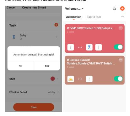
From now on, channel 1 will act as a 'pulse' contact: every time it is activated, it will deactivate after 2 seconds, regardless which input the channel activates (transmitter and TUYA app).
