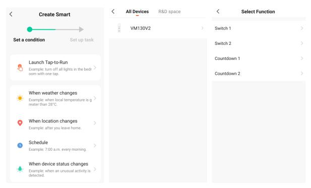
Select the on option (ON). Next, select the "Delay" task and a delay time of 2 seconds.
