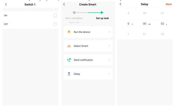
We have an overview of the set 'smart' action. Now, the channel needs to switch off after the set delay. For this, we add another task, where we select "Run the device" and device VM130V2.
