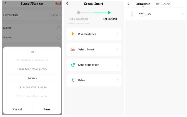
Now, we select the desired channel we wish to switch at sunrise, in this case channel 1 (Switch 1). Select the 'ON' option. Finally, we have an overview of the selected parameters. Click on 'Save'. From now on, channel 1 will switch at sunrise. You can always activate/deactivate this smart action via the 'Smart' tab.
