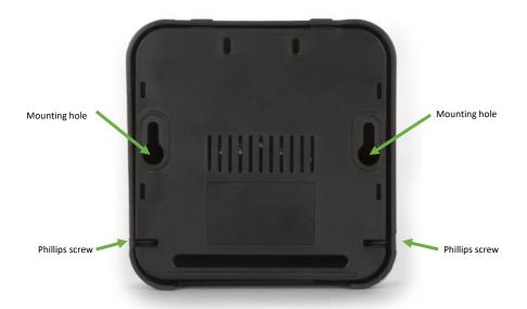
The receiver can easily be mounted against a wall or ceiling with the 2 mounting holes in the back of the case. The mounting holes have a diameter of 6,3 mm and the centre points are 62,9 mm apart from each other. Loosen the 2 Phillips screws on the two sides of the case to open the enclosure.
