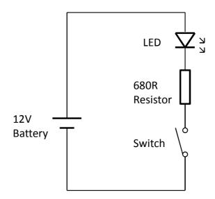
The circuit diagram for the torch is shown above. It is a very simple circuit, powered by a 12 Volt battery.
