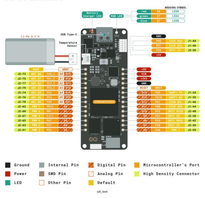
Detailed information on the Portenta H7 Lite's pinouts are available in a separate document: https://content.arduino.cc/assets/Pinout-PortentaH7\_latest.pdf
