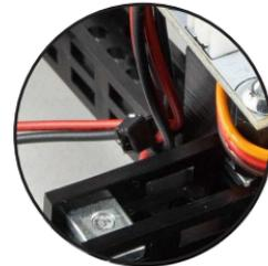
Tie wires with Zip Ties so they do not hang messy and Gripper part can move freely.
