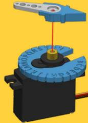
5. Place the servo arm so that the index arrow would point to letter B on the index disc. All motors are slightly different so the arrow might be not exactly on point.
