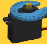
3. Carefully take off the arm and place the index disc on the motor
