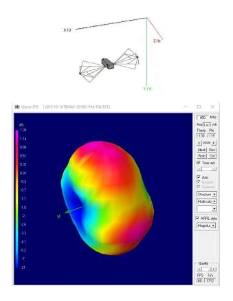
radiation pattern of the TBMA1 at 450 MHz
