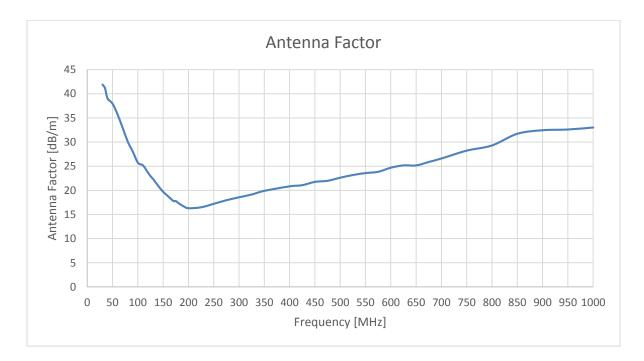
30 MHz...1 GHz , Antenna Factor of TBMA1
