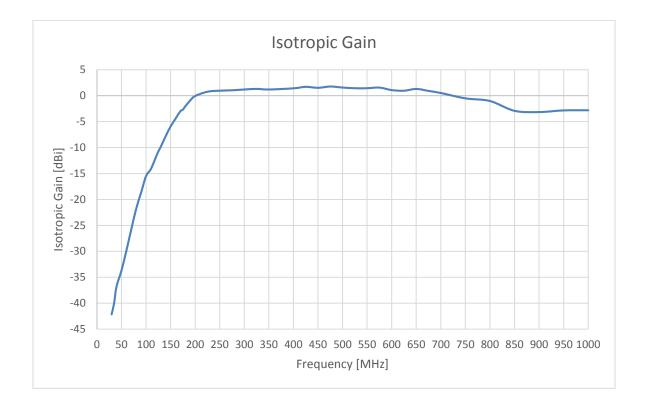
30 MHz...1 GHz , Isotropic Gain of TBMA1
