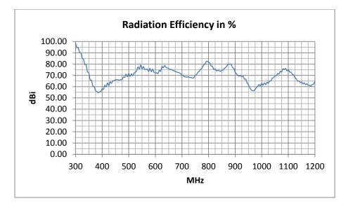
300MHz...1200MHz , TBMA1 Radiation Efficiency
