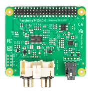
Raspberry Pi DAC+ is a high-performance audio HAT compatible with any Raspberry Pi computer that has a 40-pin GPIO header. With the Texas Instruments PCM5122, it delivers stereo analogue audio to a pair of phono (RCA) connectors. It does not require external power, and connects directly to Raspberry Pi's GPIO header with no need for soldering or cables.
